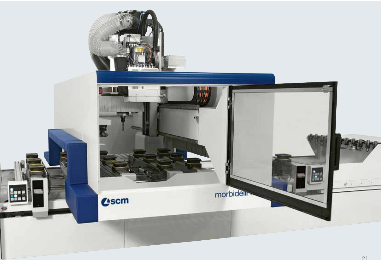
Rapidity and ergonomics to equip and do maintenance to the operating group thanks to the practical frontal opening.
