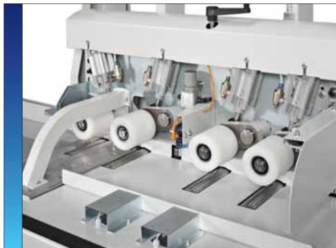
Working table with double marking station
